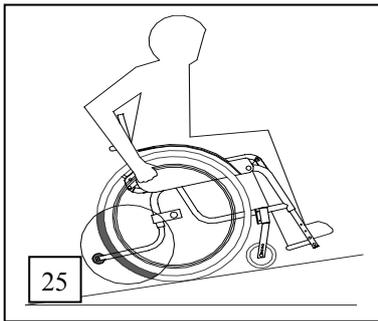
As an additional safety measure you can fit anti-tip rollers (see photo 25). We recommend to permanently fit such rollers. Attention: If anti-tip rollers are required, check that they are fitted in extended position!
