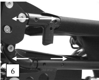
The seat depth is adjustable and grows like that with your child. It is changeable in 6 various positions from minimum 24 cm to maximum 35 cm, in distances of 2.25 cm (see photo 6).
