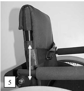
The armrests are adjustable and can through moving on the backrest be infinitely variable changed from 10 cm by the seat support to maximum 22 cm (see photo 5).
