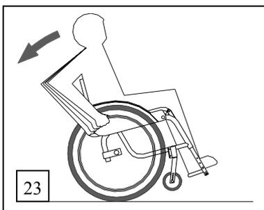
Always remember that when pushing the wheelchair on the handrings the front castors will loose traction due to acceleration. Depending on the weight distribution, this may cause the castors to lift off the ground and the wheelchair to tip over backwards (see diagram 23).
