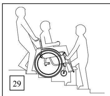
They should under no circumstances take hold of any moving parts, such as the wheels or armrests (see diagram 29). Always ensure that the stroller handle is securely fastened with the clamping levers.
