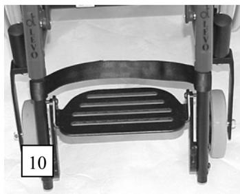
The calf/heel strap serves to prevent the legs and/or feet from slipping backwards. The calf strap is fitted to both leg support tubes and fixed using a Velcro fastening (see photo 10). The calf strap should be fixed that it is just touching your heel or calf when your feet rest on the footrest in the seating position. Because of the Velcro fastening it can be adjusted in the length so that the feet are in the ideal position. This is very important for a good standing position.
