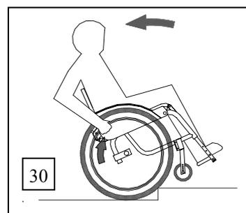
If the child wants to overcome an obstacle alone you should be aware of the tendency of the wheelchair to tip over backwards if, as the rear wheels contact the edge of the obstacle, the child attempts to surmount it by pushing down harder on the handrim (see diagram 30).
