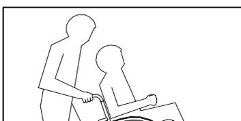
To descend over an obstacle (e.g. driving down from the kerb into the street), first tilt the wheelchair up onto the rear wheels, push it forward and let the wheelchair down over the edge of the obstacle on two wheels (see diagram 28).
