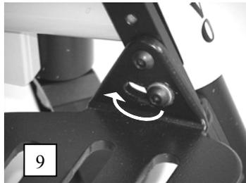
The footrest is in an angle of 90° to the leg support. This means an angle of 20° with the floor (backward inclination). The footrest is also in the angle adjustable by plus/minus 5° (see photo 9).
