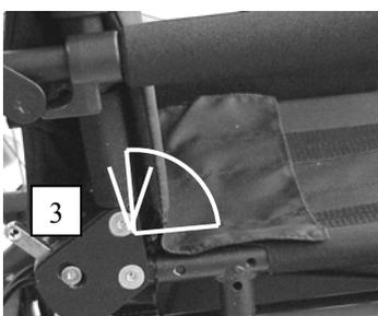
The standard pre-set angle between the backrest and seat is 90°. It is possible to re-set this angle either by 5° further forward or 5° further back.
