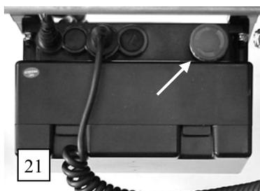
Trough pressing the red emergency cut-out switch on the right side of the battery box the circuit will be interrupt and it will stop the lifting of the seat in the case of an emergency (see photo 21). You can switch on power again, by turning the red emergency cut-out switch clockwise. The standing mechanism is again ready to use.
