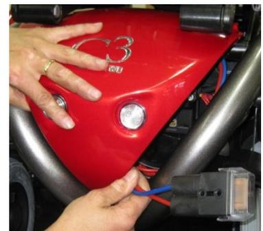
The main fuse housing is under the chair cover in the rear. To get access, carefully open the cover as shown above.
