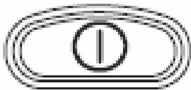
With the On-/ Off-button the chair can be turned on or switched off. Don't use this button to stop the wheelchair, unless there is an emergency.
