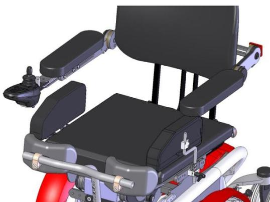
Leads the thigh and stabilizes the leg axle in seating and standing position. Can be adapted individually in place, distance, angle and height. To change the position, open the zipper at the outside of the pad and untighten the screws lightly, now you can adjust the pad to the necessary position, tighten the screws afterwards.
