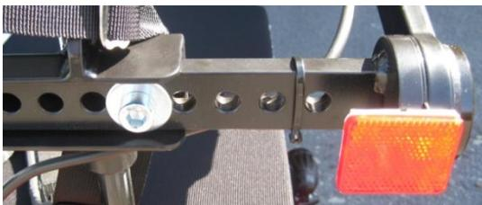
Untighten the two screws. Now you can adjust the armrests in the width.
